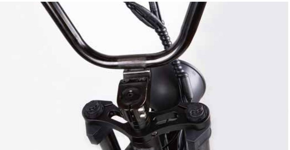
3. Center the handlebar and tighten the bolts on stem faceplate evenly.
