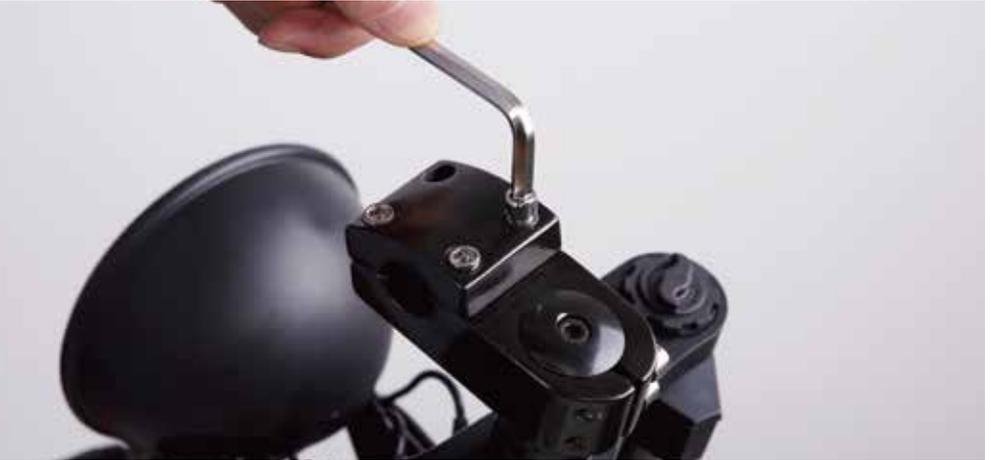
2. Place the handlebar on the stem correctly. Trace the front brake cable directly up from the front brake caliper to the left handlebar and ensure the cables and wires are not twisted. **Notice:** The horn is on the left hand side and the gear shift is on the right.
