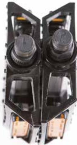
2. The right pedals threaded to tighten by turning clockwise. The left pedals reverse-threaded and tightens counterclockwise. Carefully thread the pedal onto the crank by hand slowly.
