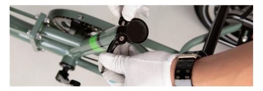
2. Insert seat post into seat tube. Adjust the seat post up or down to a comfortable height, while ensuring the seat post is inserted into the frame past the minimum insertion point.
