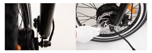
4. Once the lock washers are in place tighten both axle nuts with the supplied double-open end wrench.
