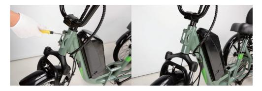
2. Assemble the front basket. The 4 holes of the basket are aligned with the 4 holes of the frame, use the screwdriver to assemble it with front basket screws.
