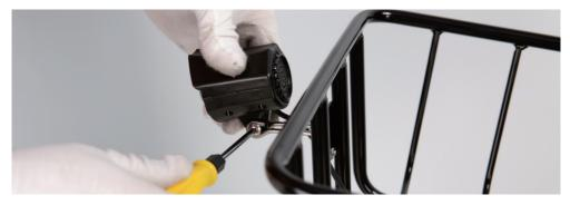
2. Fix the headlight cable. Fix the headlight cable to the bottom of the basket with a zip tie. Then cut off the excess part of zip tie.
