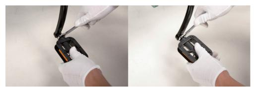
3. Further tighten with the supplied double open-end wrench. Do not cross thread or damage the threads.
