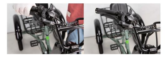
Cancel the parking function: Hold the brake handle and pull up the parking button to cancel the parking function.
