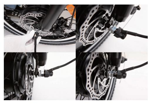
3. After inserting the front axle onto the fork, you will need to line up the axle lock washers (these are the metal washers, put thin one on the inside, thick one on the outside) with the hole at each fork.
