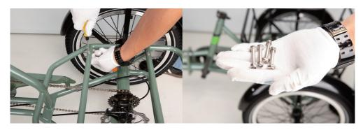
2. Align the 4 holes of the rear basket with the 4 holes of the rear frame, with an even distance between the left and right, and put back the mounting bolts, tighten it with screwdriver.
