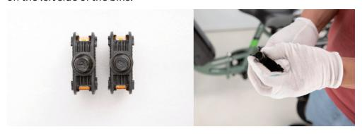
2. The right pedals threaded to tighten by turning clockwise. The left pedals reverse-threaded and tightens counterclockwise. Carefully thread the pedal onto the crank by hand slowly.
