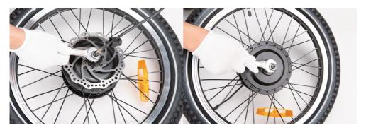
2.Lift the front of the bike and lower the fork onto the wheel axle. Notice: The brake rotor should go into the brake caliper in between the brake pads and the axle should enter the fork dropouts fully. The front rotor orientation should be to the left of the fork.
