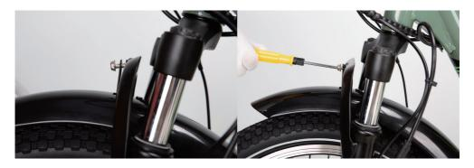
3. Tighten with the screwdriver.
