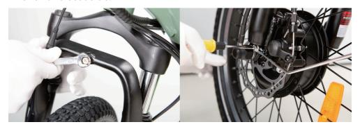
2. Place the fender in position. Pass the front fender mounting point under the front fork arch from the back of the front tire.
