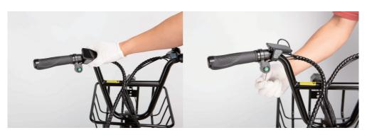
6.Hold the brake tightly and press the parking button when stopping the ebike, the brake is locked to start the parking function, the ebike will not move.
