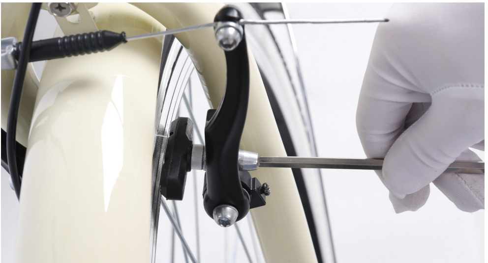
2.Cable Attachment. Before we draw the pads together, back out the barrel adjusters three or four turns. So that we can have some fine tuning at the lever.
