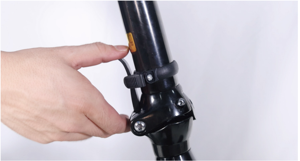
(4).Tighten the bolt in the center of the stem with the supplied allen wrench.
