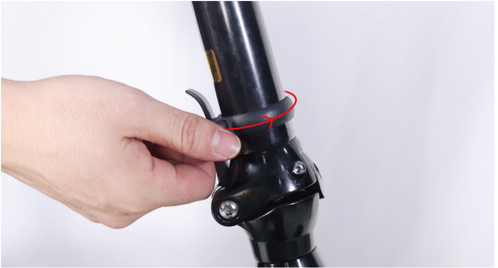
(3).Unfold the quick release lever downward to open the stem.
