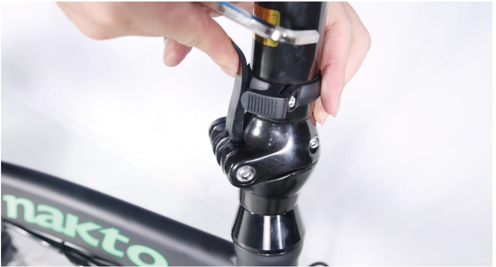
(6).Turn the plastic clasp clockwise to secure the quick release lever.
