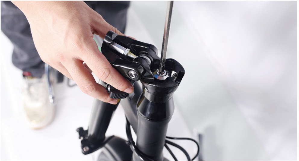
(5).Close the quick release lever to secure the stem.
