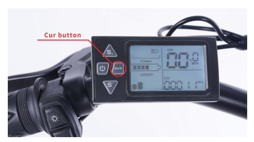
5.**Select the desired level of pedal assistance**—Select the level from 0-5 by pressing "S+" and "S-". Level 1 corresponds to the lowest level of pedal assistance, and level 3 corresponds to the highest level of pedal assistance. Level 0 indicates pedal assistance is inactive. Start in PAS level 0 or 1 and adjust from there.
