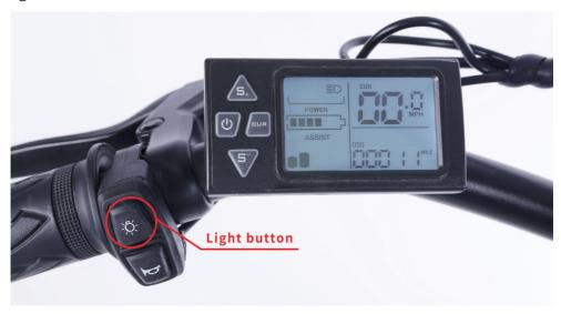
(2).Once the LCD Display is on, press "CUR" button to turn the headlight on. Press it again to turn the headlight off.
