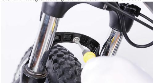
2.Attach the headlight to the fork arch. Pass the bolt through the headlight mount and fork arch mount. Tighten with the supplied screwdriver.
