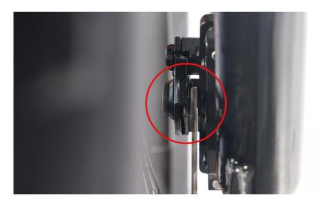
3.Tighten both axle nuts with the supplied double-open end wrench. **Noteic:** Before doing the final tightening of the axle nuts, make sure the wheel is square and true with the forks.
