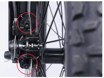
If the pads are still rubbing, we need to do some fine-tuning. Loosen one bolt at a time and adjust until there is a gap on either side of the rotor. Once the pads are not rubbing, fully secure each mounting bolt and the process is complete.
