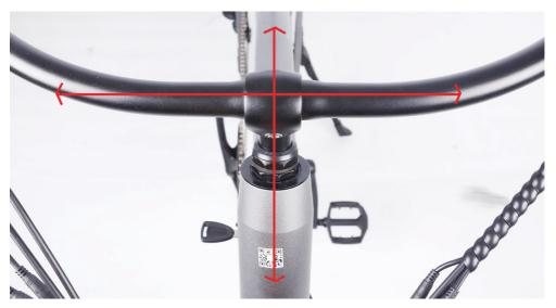
4. Tighten the bolt on top of the handlebar stem with the supplied allen wrench.
