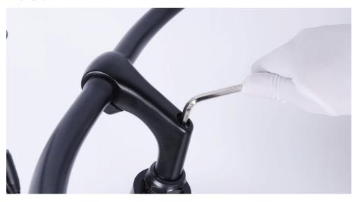
5.Use the supplied allen wrench to loosen the handlebars angle adjustment bolt, tilt the handlebars to the optimal position, and tighten in place securely.
