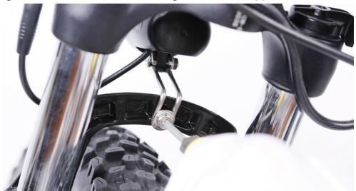
3.Center the headlight and adjust the angle slightly downwards to illuminate the road ahead and not blind oncoming traffic. Use the supplied Phillips-head screwdriver to loosen the headlight angle adjustment bolt, tilt the headlight to the optimal position, and then tighten in place securely.
